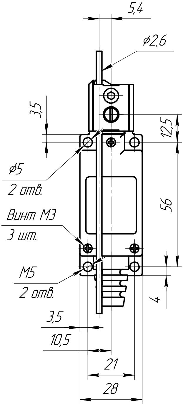
Technical drawing showing a cross-sectional view of a cylindrical component. Key dimensions include: top width 5,4; top hole diameter  $\phi 2,6$ ; side hole diameter  $\phi 5$  with 2 clearance holes; side height 3,5; side width 10,5; side height 21; side width 28; side height 3,5; side width 12,5; side height 56; side width 4.
